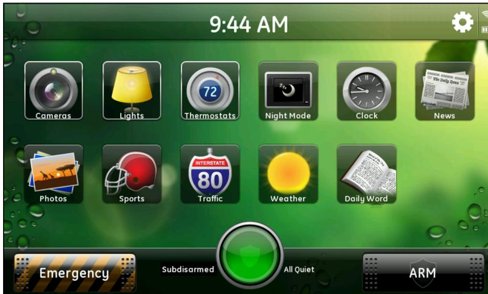
To reverse the subdisarm (that is, to re-arm the special items but leave the rest of the system disarmed), return to the Home screen and touch **DISARM**. No access code is required to disarm the system in this situation. The security system returns to the disarmed state.
