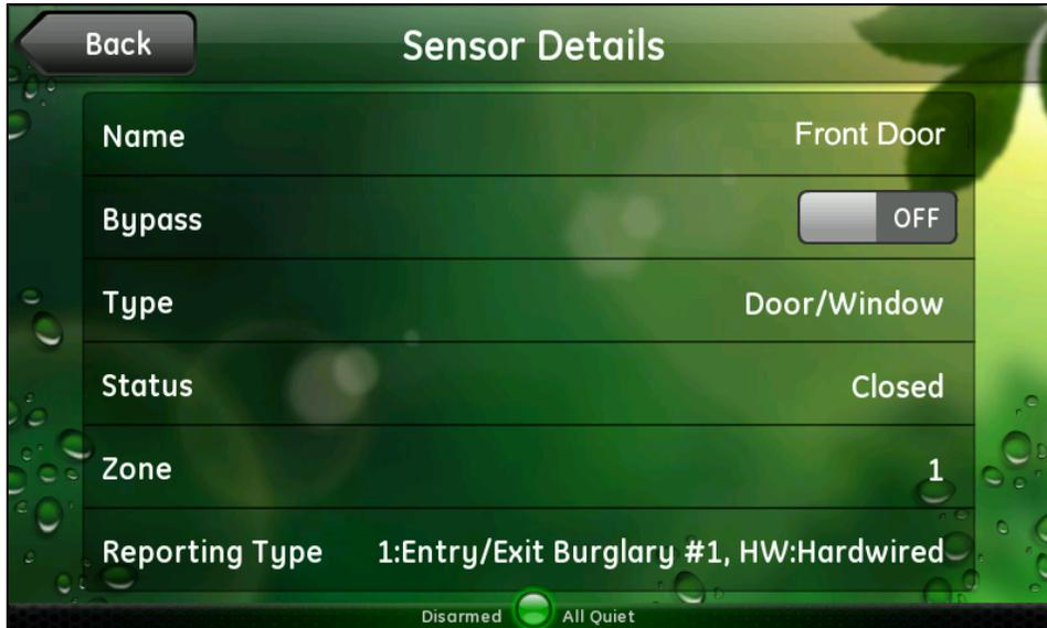
The Sensor Details screen provides information about the selected sensor. You can touch Bypass to turn on bypassing for this sensor. (See ["Bypassing Sensors" on page 16](#) ["Sensors" on page 14](#) for details.)
