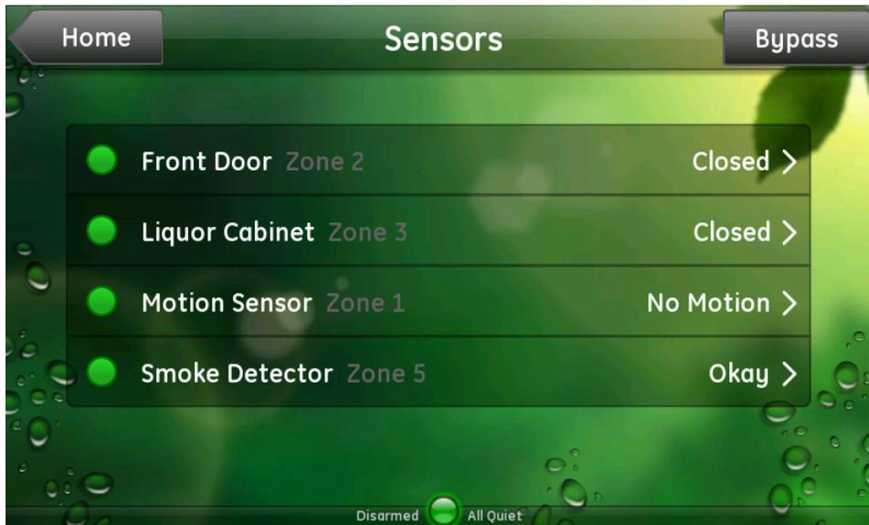
This screen displays a list of all sensors installed at your site and the current status of each. You can:
