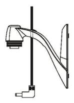
• Screw/attach the camera onto the camera stand.
