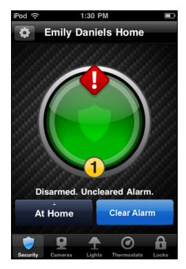
If you have an uncleared alarm, before performing other security panel functions, you must specifically clear the uncleared alarm by tapping **Clear Alarm**.
