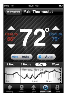
The currently selected mode appears below the temperature display. The mode setting indicates whether the thermostat is controlling heating, cooling, both (**Auto**), or is turned off. To change the mode, tap the mode button to view the list of modes, then tap the desired setting.
