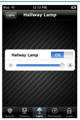
The **ON/OFF** selector shows the current state of the light, and can also be used to change the state. A light that is on shows "ON" on a blue background, whereas a light that is off shows "OFF" on a gray background.
