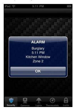
Tap **OK** to acknowledge the dialog. At this point, the alarm is still active, and the "Alarm" system icon displays.
