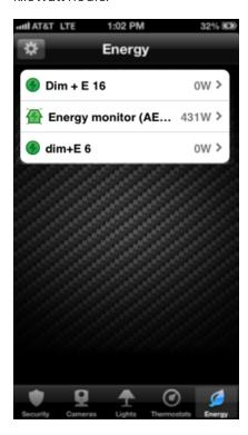
The icon to the left of the name indicates the type of energy monitor device and its state.
