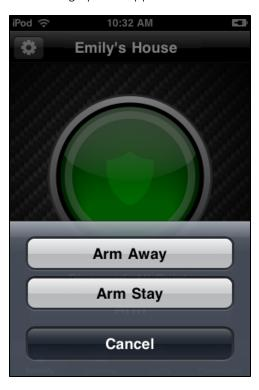
2. Tap Arm Stay to arm perimeter sensors only, or tap Arm Away to arm all perimeter and interior sensors.
