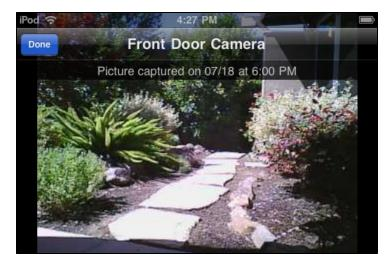
The picture screen displays the name of the camera, the date and time the picture was taken, and a **Done** button as an overlay. After a few seconds, the overlay disappears, and only the picture is displayed. You can tap the screen to display the overlay again.
