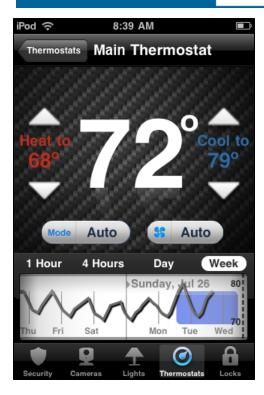
If the temperature goes above the thermostat's cool setpoint, a blue area on the graph indicates when the air conditioner was activated. If the temperature goes below the thermostat's heat setpoint, a red area on the graph indicates when the heat was activated.
