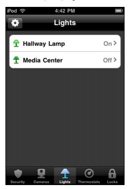
The Lights list screen shows all of the switches installed at your site, and the current state of each (on or off). The icon to the left of the name also indicates the state.
