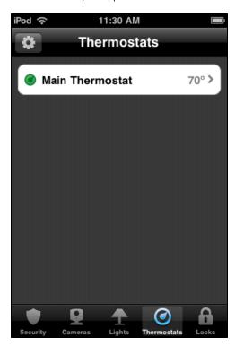
The Thermostats list screen shows all of the thermostats installed at your site, and the current temperature at each thermostat's location. For some batteries, when the thermostat's battery reaches a low battery state, the thermostat's green icon ( ) changes to a red low battery icon ( ). In addition, when a low battery energy level occurs the system sends a system alert to indicate there is a low battery. You can tap the name of any thermostat to display details about that thermostat.
