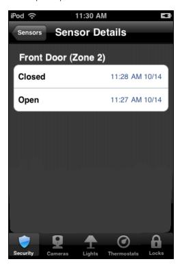
The Sensor Details screen displays the name of the selected sensor and a list of its recent activity, such as opened or closed for doors, and motion events for motion sensors.
