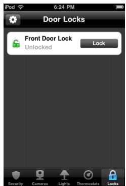
The Door Locks screen shows all of the door locks installed at your site, and the current state of each (locked or unlocked). The icon to the left of the name also indicates the state. You can use this screen to remotely lock or unlock any door. Simply tap **Lock** or **Unlock** to change the setting of any door on the list.
