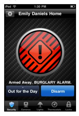
To cancel the alarm and stop the security system's alarm sound, tap the **Disarm** button.
