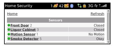
This screen displays a list of installed sensors at your site. The icons that appear to the left of the sensors indicate the status of each sensor. The following table lists all of the possible icons you might see on this screen.
